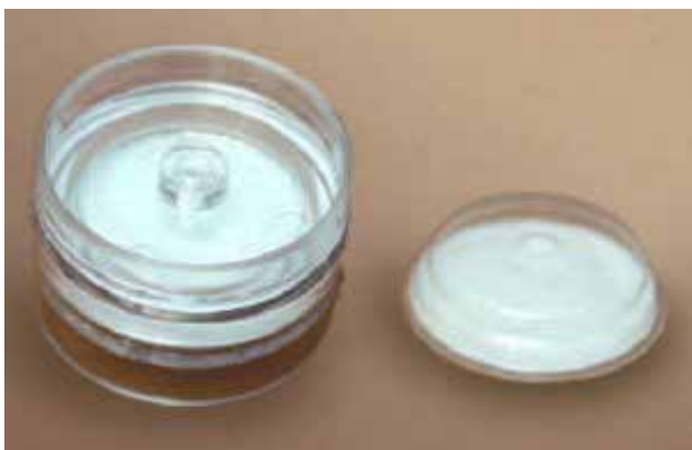
Figure 1. (a) Photograph of a 37-mm diameter plastic close-face cassette sampler (left) and an internal filter capsule (right); (b) Schematic of the CFC sampler showing placement of the filter capsule (shaded portion) and cellulose back-up pad within the cassette.
