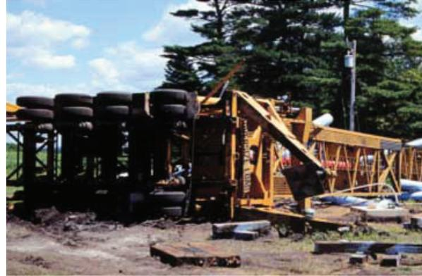
**Figure 6.** Mobile tower crane tip-over attempting to hoist water tank. (Photo courtesy of Iowa FACE Program)
