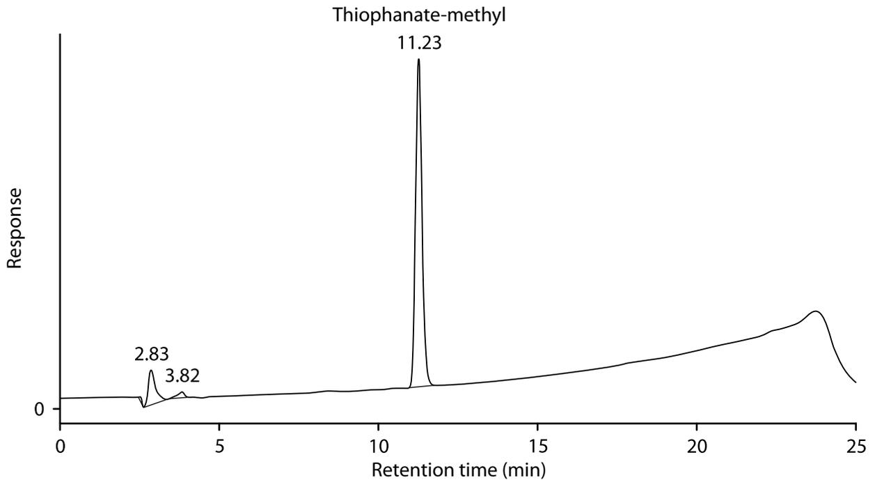
**Figure 2.** This is a typical chromatogram of a liquid calibration standard. This sample was analyzed with the Kingsorb™ column. The retention time on the Synergi™ column is 14.1 minutes.
