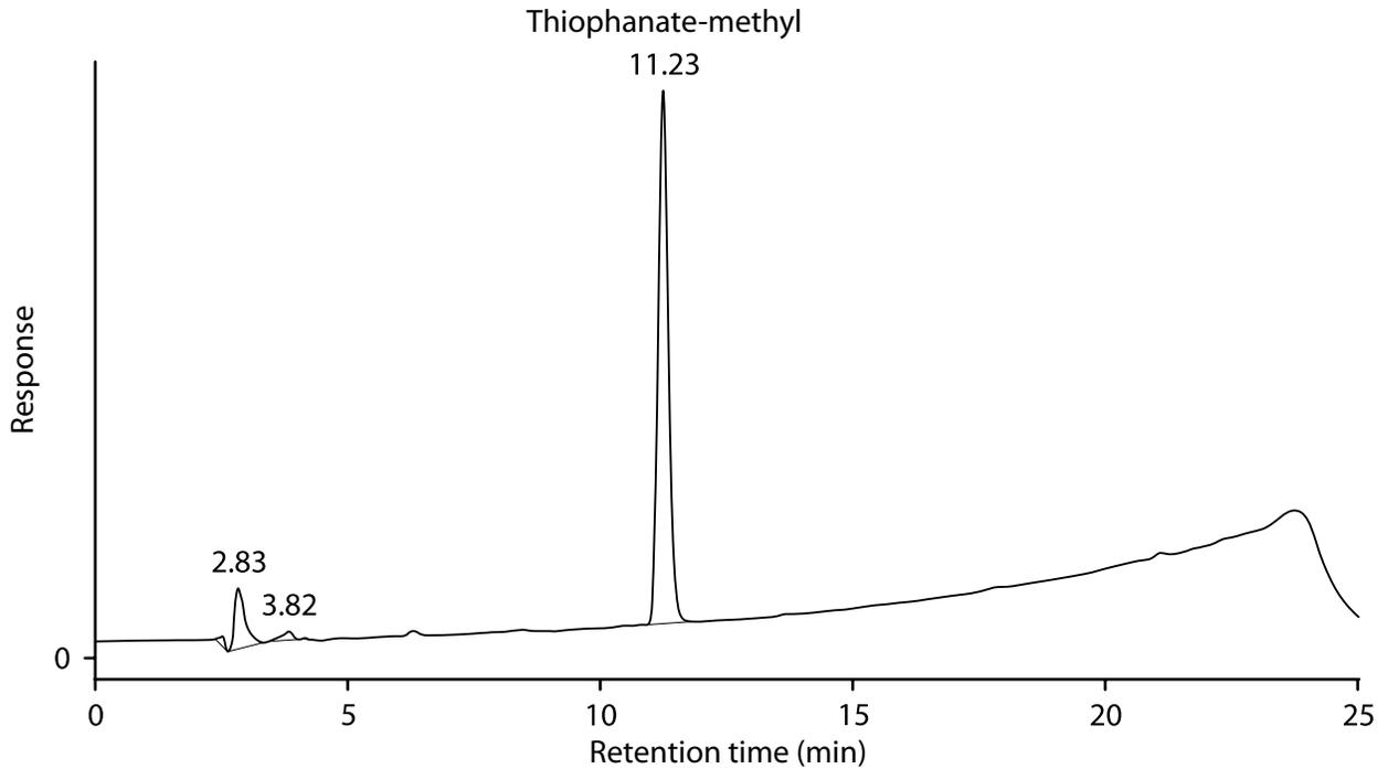
**Figure 1.** This is a typical chromatogram for a sample of thiophanate-methyl. This shows the response for a spike of 348 µg/sample of thiophanate-methyl on an OVS-2 tube, extracted and analyzed by this LC method using the Kingsorb™ column. On the Synergi™ column, the retention time for thiophanatemethyl is 14.1 minutes.
