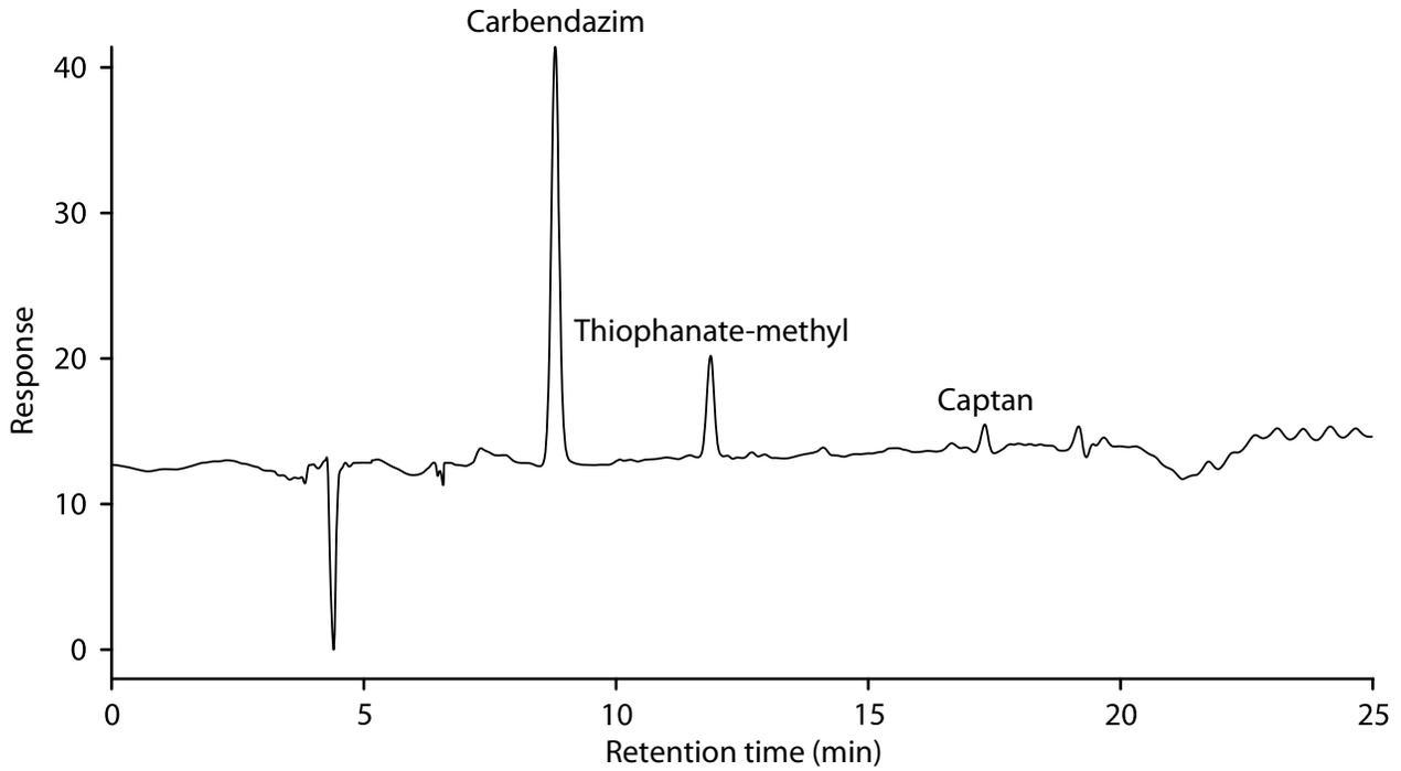
**Figure 3.** This chromatogram shows the three analytes of interest, carbendazim, thiophanate-methyl, and captan, which were extracted from a spiked OVS-2 sampling tube. This chromatogram has been background corrected by subtracting an OVS-2 blank analysis.
