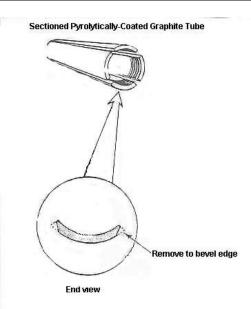
Figure 1 Construction of a laboratorymade platform.
