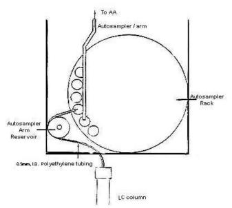
Figure 2 HPLC/AAS interface system
