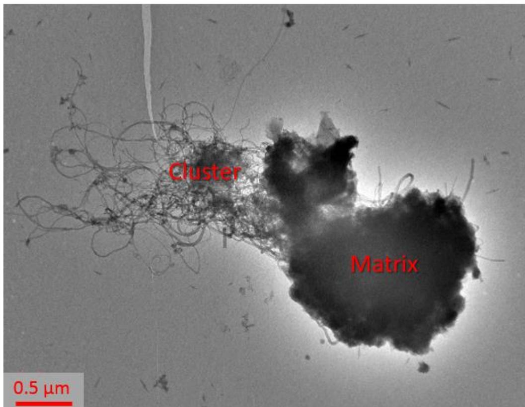
**Fig. 7.** CNT particle with both matrix (right side) and cluster (left) features. Structure categorized as a CNT matrix particle.
