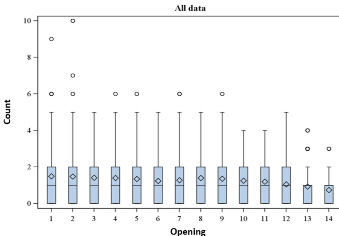
**Fig. 11.** Boxplot of CNT counts by openings (1-14). The variability in openings 1 and 2 significantly higher than that of openings 13 and 14. The means of openings 1, 2 and 3 were also higher than the means of openings 12, 13, and 14.
