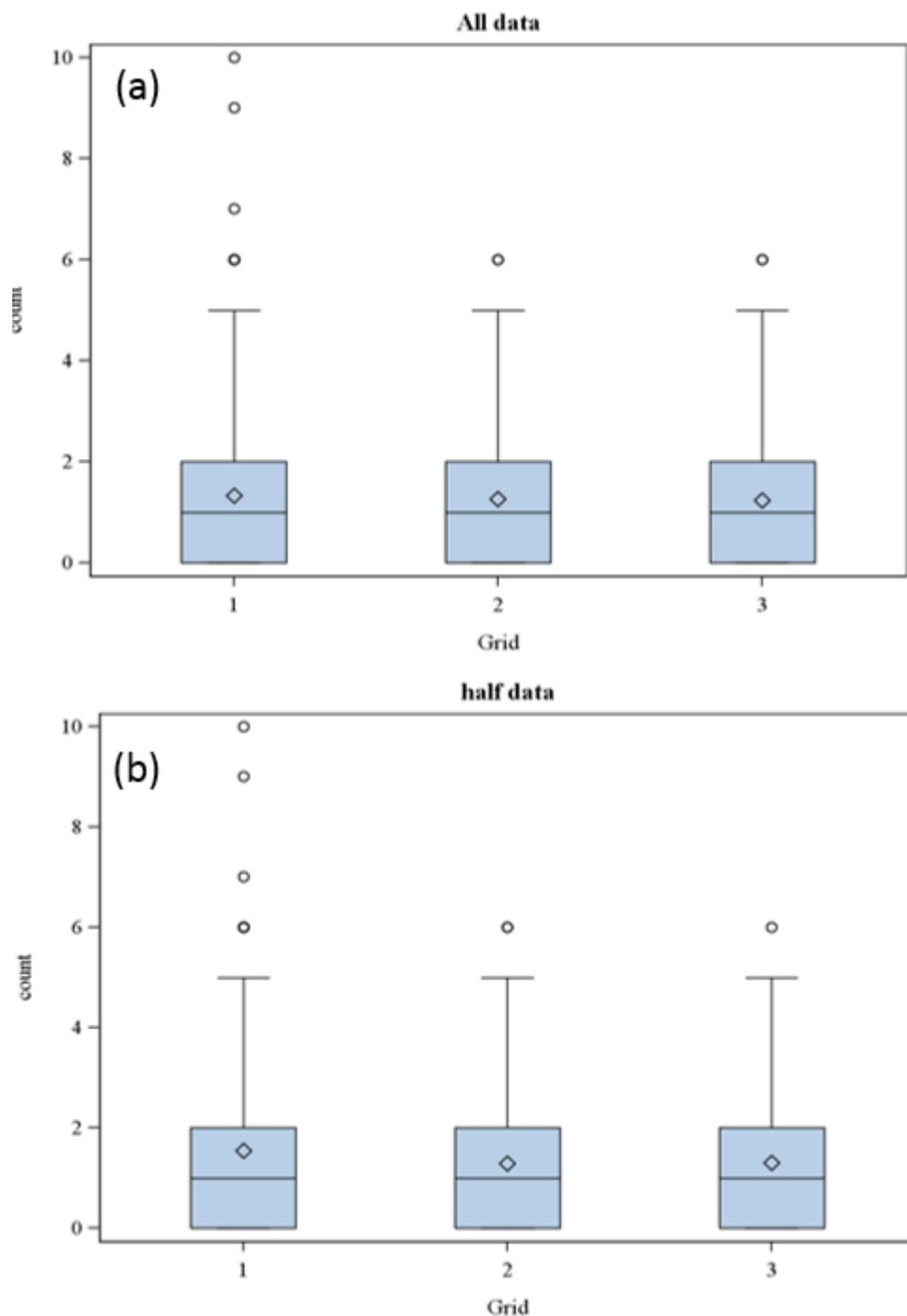
**Fig. 12.** Boxplot of CNT counts by grids (1-3) from all data (counts from openings 1-14) and half data (counts from openings 1-7).
