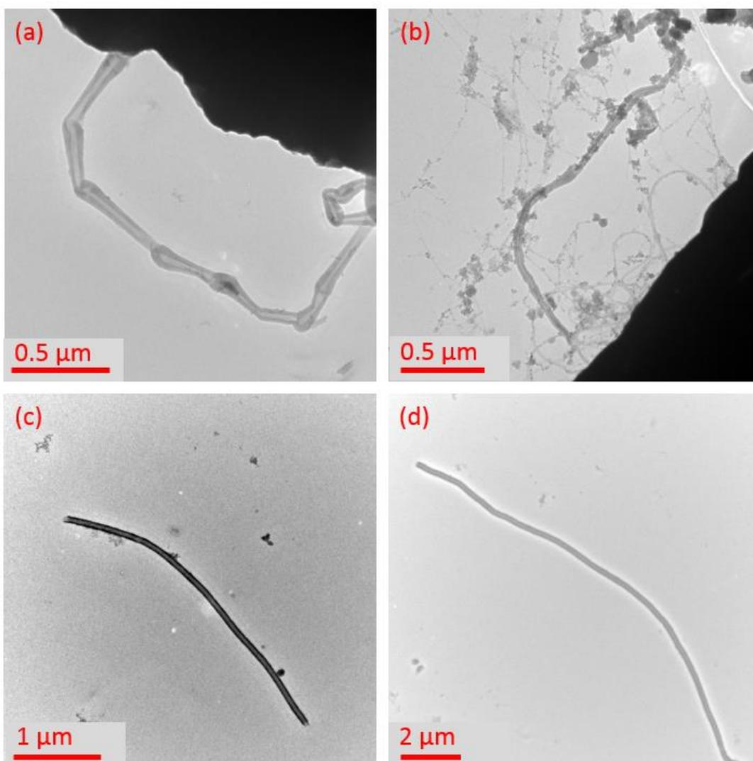
**Fig. 4.** Examples of CNT fiber structures with various lengths and widths.
