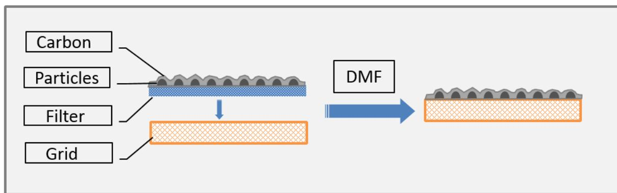
**Fig.3.** Removal of residual MCE polymer from carbon-coated sample by dimethylformamide (DMF). After polymer removal, only particles embedded in the carbon film remain on the grid.
