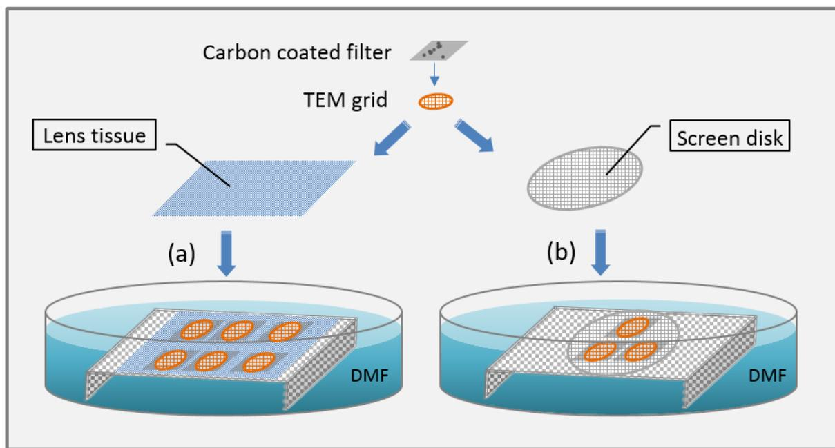
**Fig. 2.** Sample transfer and final processing: place a piece of lens tissue (a) or a stainless steel screen disk (b) on a stainless screen platform in a Jaffe wick washer filled with dimethylformamide (DMF). Sides of the platform are bent to keep sample grids above the solvent level. Depending on size, multiple disks can be used to hold grids.
