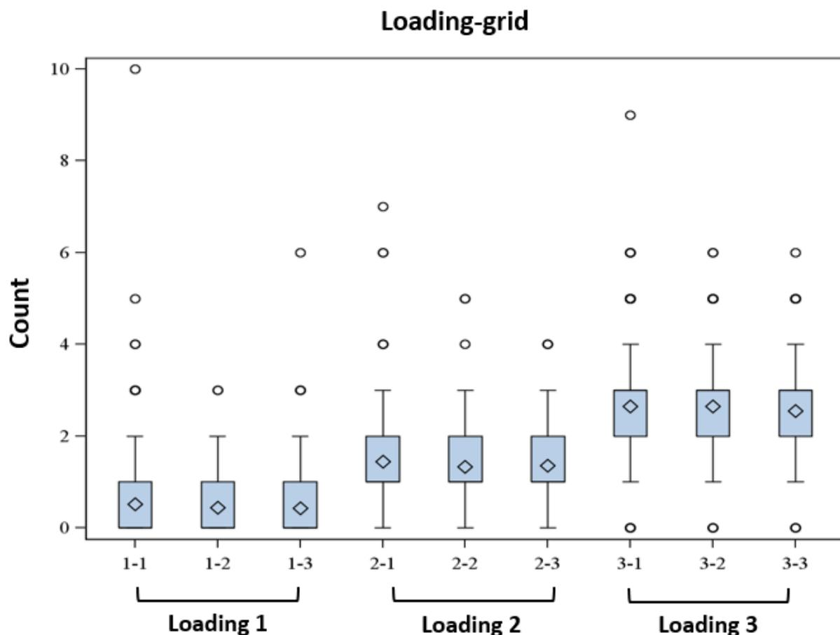
**Fig. 10.** Boxplot of CNT counts by categorized loading (1: mean  $\leq 1$ , 2:  $1 < \text{mean} \leq 2$ , and 3: mean  $> 2$ ) from three grids. The trend of mean counts from grid 1 to 3 is consistent for different loading levels. Mean count of grid 1 is slightly higher than those of grid 2 and 3.
