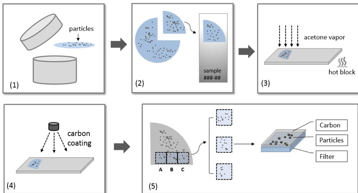
**Fig. 1.** Filter preparation steps prior to loading sample portions on TEM grids: (1) remove 25-mm MCE filter from air sampling cassette; (2) remove about one fourth of the filter and place the filter wedge on a glass slide; (3) clear the MCE filter with acetone vapor in a hot block; (4) apply carbon coating; (5) cut section from coated filter and divide into three portions, one per grid. Each filter portion has particles sandwiched between the carbon film and collapsed filter.
