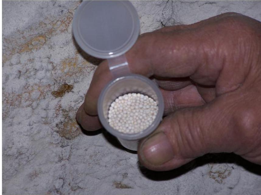
**Figure C1. Sample tube containing molecular sieves.**
