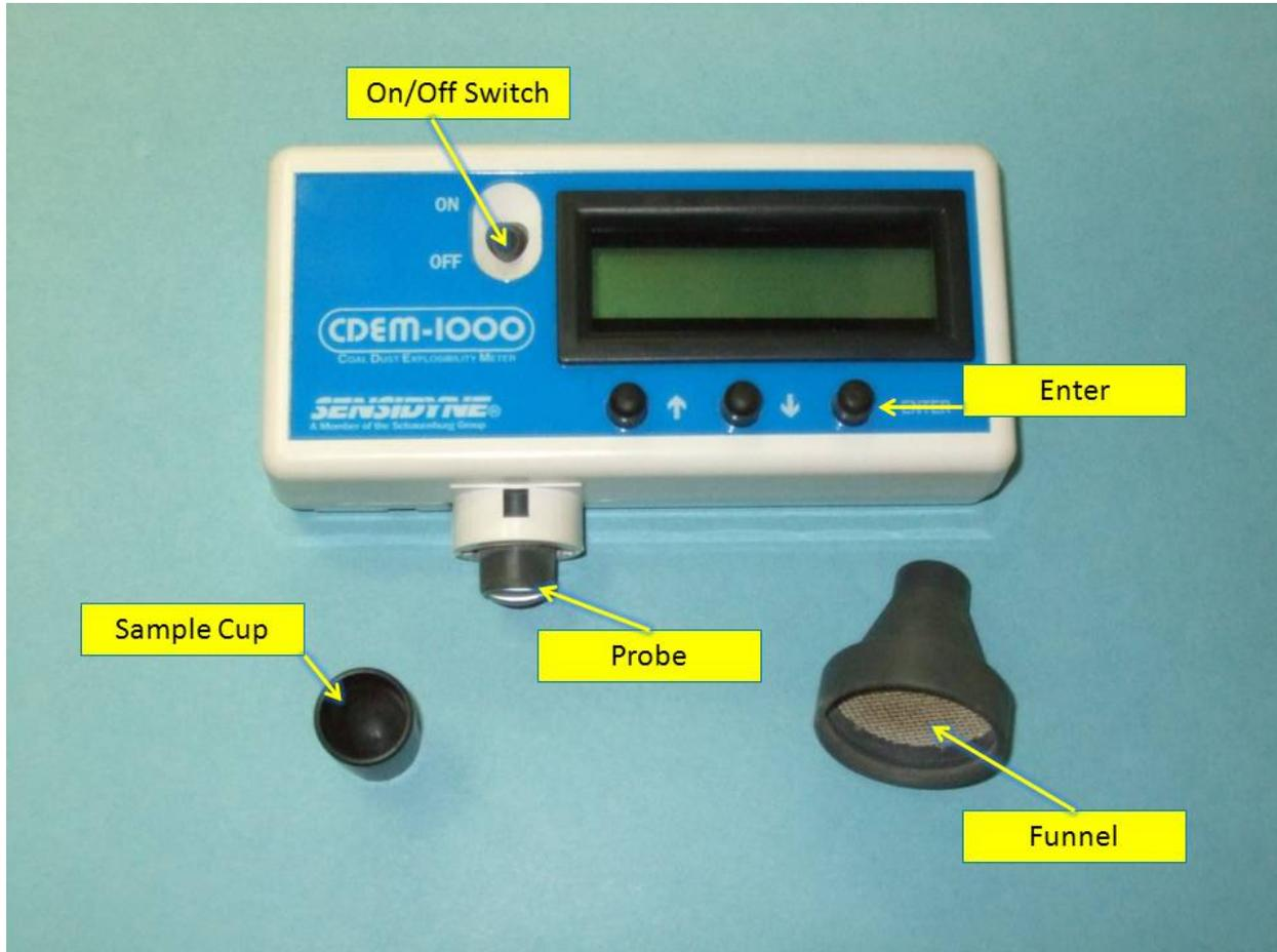
**Figure A1. Coal Dust Explosibility Meter (CDEM).**
