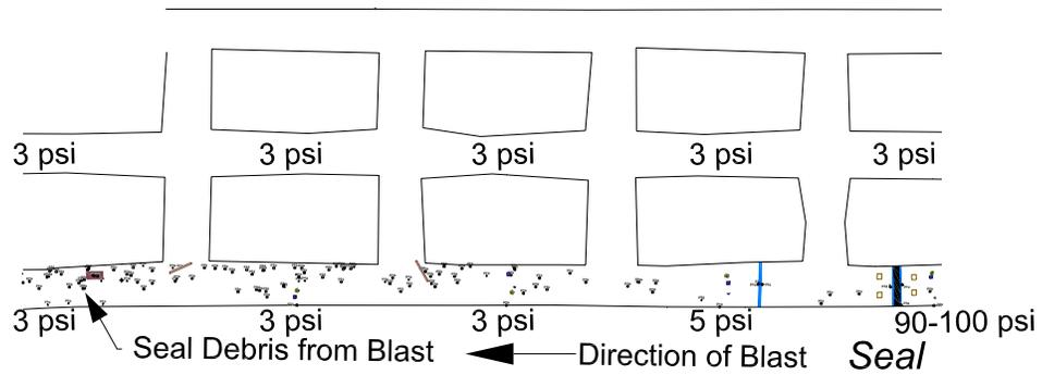
Figure 2 – Most debris from an explosion remains in entries parallel to the direction of the blast. Little debris affects entries perpendicular to the blast. Locate refuge chambers in cross-cuts at right angles to the most likely “line of fire” from an explosion to protect the refuge chambers from projectiles.
