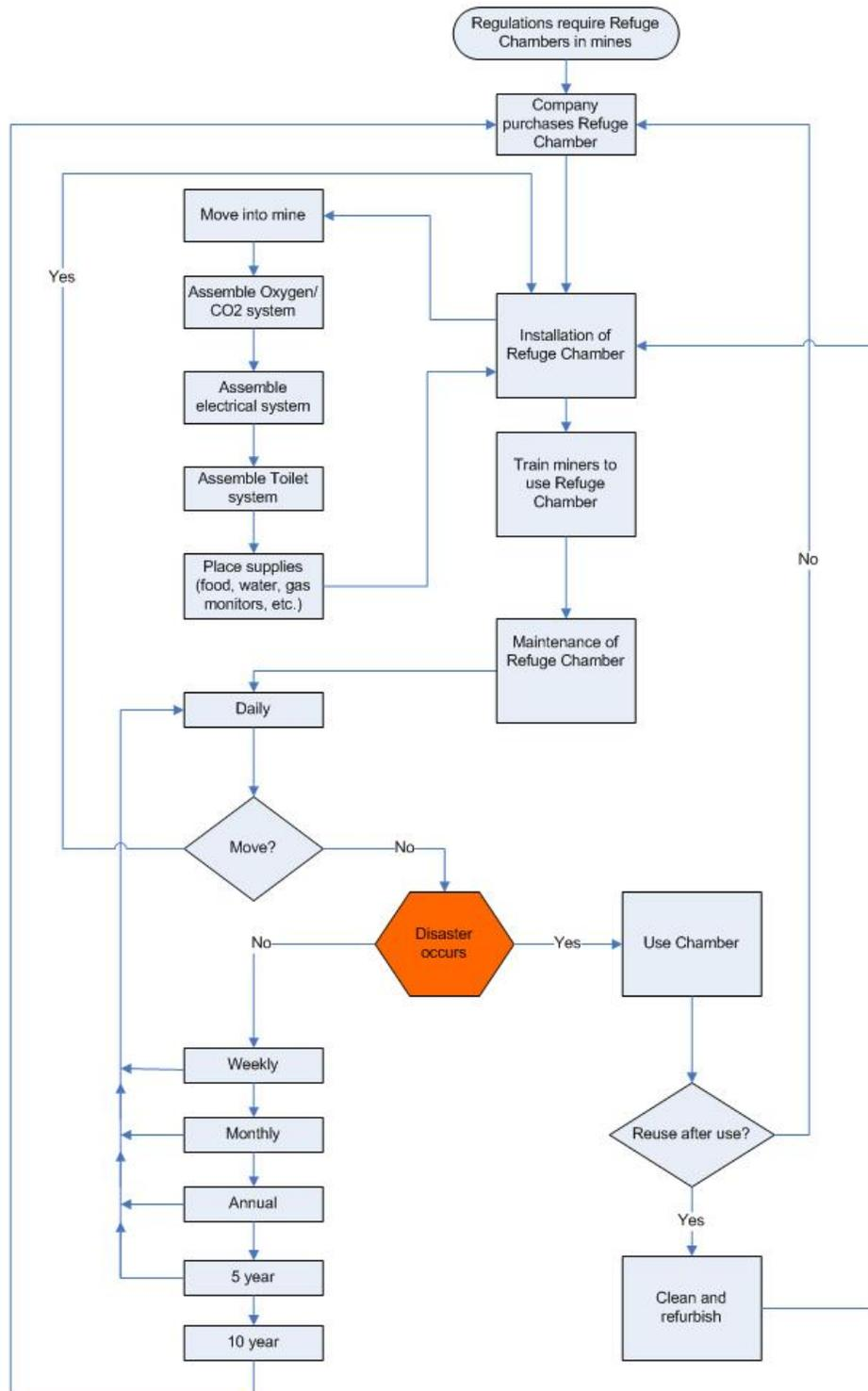
**Figure 1. Flowsheet presenting steps for implementation of a portable refuge chamber.**
