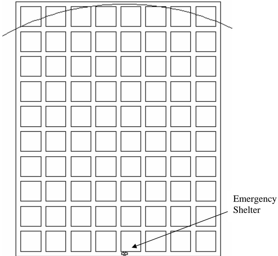
**Figure A2. Area available for mining for 9 entry system: Arc is limit for 1000 ft distance away from face assuming linear advance.**
