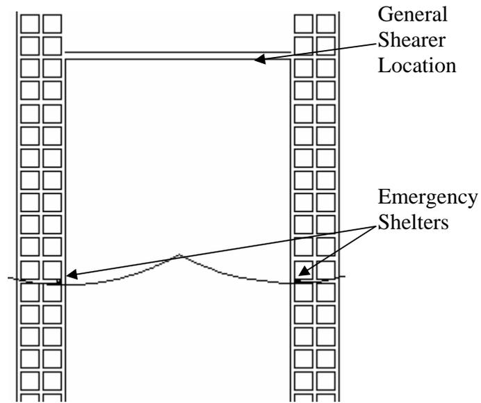
**Figure A3. Area available for mining for longwall system: Arcs are limits for 1000 ft distance away from face assuming linear advance.**
