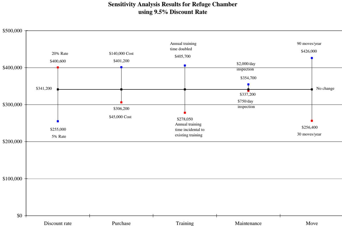
**Figure 2. Summary of sensitivity analysis completed on refuge chamber costs.**
