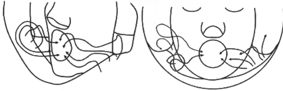
Figure 4. Simplified diagram of fog across the face when the Centurion blower was producing 100L/min and the breathing flow was higher. Each figure depicts a different layer of fog flow within the visor and head form that was only visible when inhalation flow exceeded blower flow.
