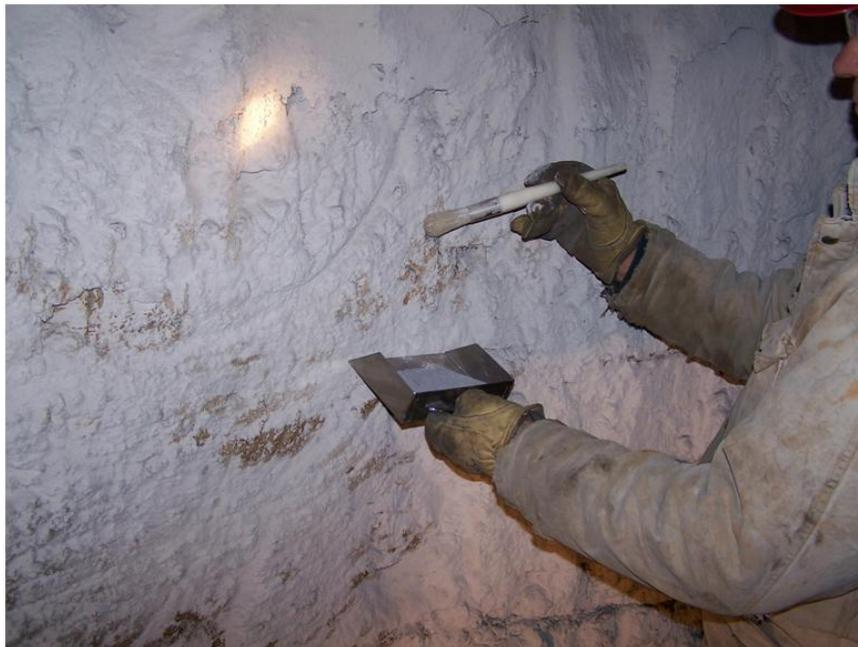
**Figure C2. Collecting a band sample.**
