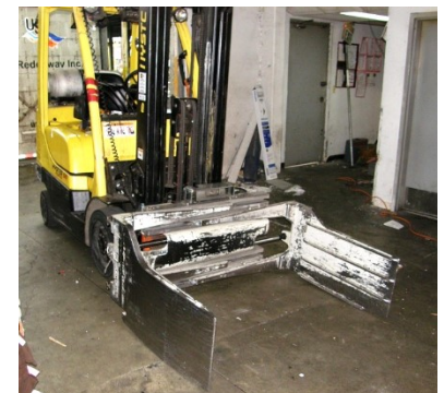
Photo 2: Incident forklift with bale clamp attachment.
