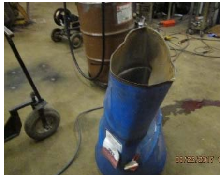
Photo 4. View of damaged drum following explosion; bottom of drum was blown off. (Photo courtesy of OR-OSHA)
