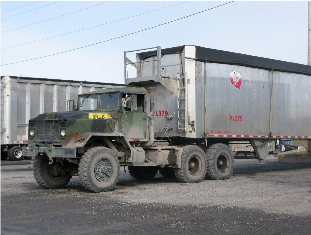
Photo 4. A military surplus tractor (“army truck”) was used to haul the trailer and deposit waste in the landfill.
