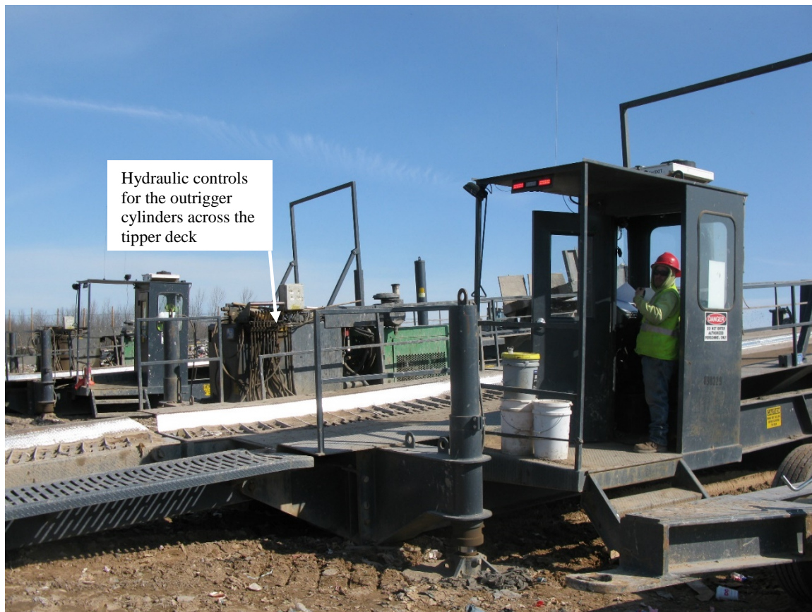
Photo 2. Hydraulic controls for the outrigger cylinders were on the left side of the deck and the operator's cab was on the right side.
