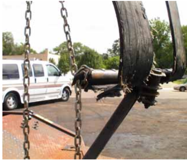
Figure 3. Wrapped tow chain on lifter bar grab hook
