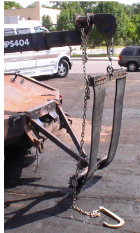
Figure 4. Completed tow chain securement to tow truck after chain fed through “O” ring on tow mast
