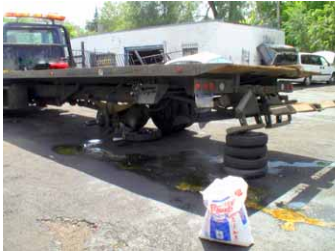
Figure 5. Tires used as improper primary support
