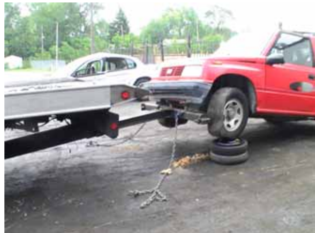
Figure 10. Use of tow vehicle to raise vehicle and improper secondary support for a different vehicle on the employer's worksite
