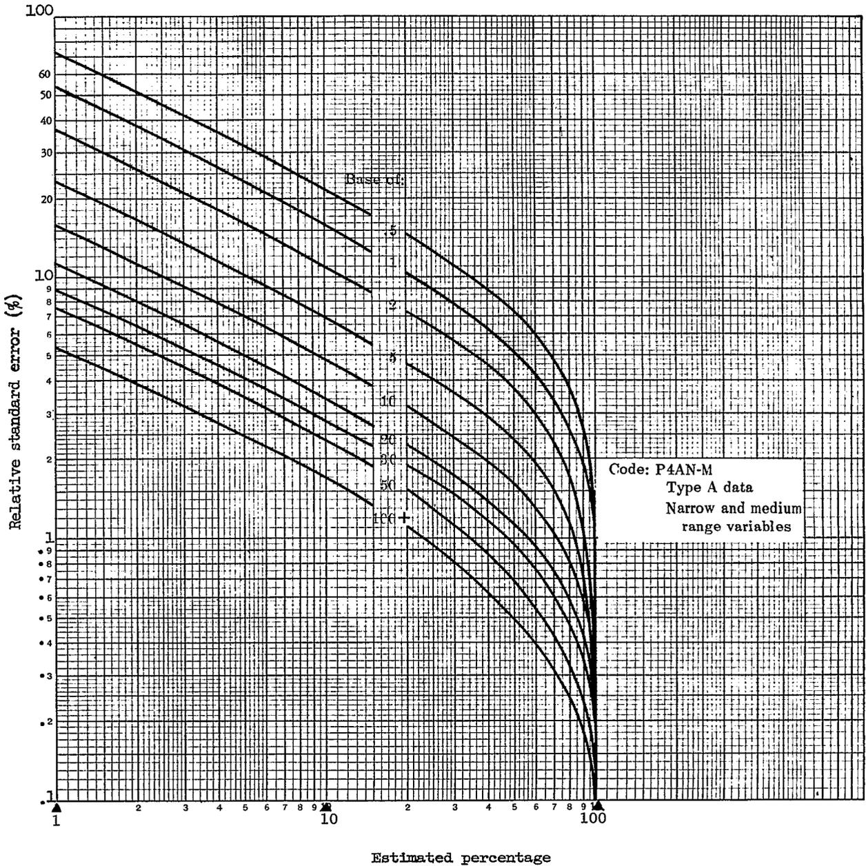
Example of use of chart: An estimate of 20 percent (on scale at bottom of chart) based on an estimate of 10,000,000 has a relative standard error of 3.2 percent (read from the scale at the left side of the chart), the point at which the curve for a base of 10,000,000 intersects the vertical line for 20 percent. The standard error in percentage points is equal to 20 percent X 3.2 percent or 0.64 percentage points.
