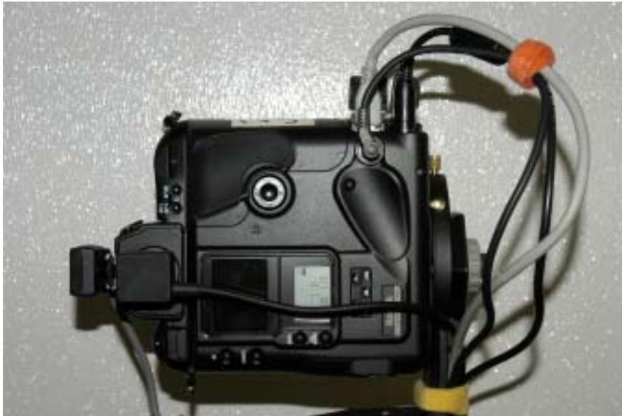
Use two additional ties to secure the cables near the LCD monitor and between the LCD monitor and the camera. Optionally, place a tie around the cables extending from the adjustable arm to the wall.
