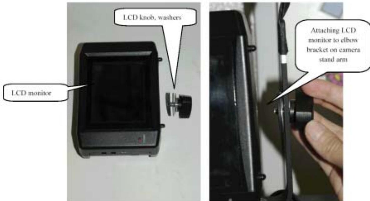
Connect the LCD monitor to the mini-camera as follows: note that the minicam-LCD cable extends from the mini-camera to a cylindrical-shaped power plug and splits at the end into two small cords with a male and female plug. Insert the female plug in the DC IN 12V port on the LCD monitor. Insert the male plug into the AV IN port. The ON/OFF switch for the LCD monitor is located beside these ports.
