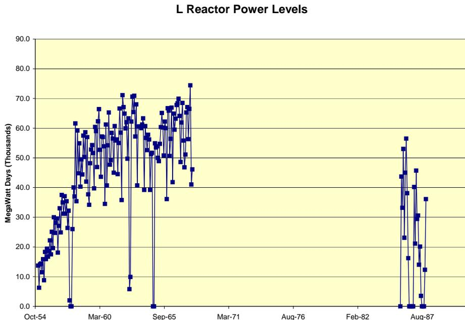
**Figure 2-7.** L-Reactor operated from 1954 through February 1968, reaching its maximum monthly output of 74,400 MWD in December 1967. It operated again from November 1985 through December 1987. A January 1960 rapid restart lead to a serious incident in which fuel temperatures could have reached the melting point. SRS procedures were modified to prohibit rapid restarts as a result of that incident ([Du Pont XX](#)).
