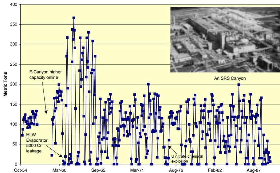
**Figure 2-11.** F-Canyon uranium to dissolver. The first plutonium extraction at SRS took place in November 1954 in the F-Canyon. The canyon reached its peak capacity in April 1962. A leak from a HLW waste evaporator in mid-1960 caused internal flooding and contamination ([Du Pont XX](#)).
