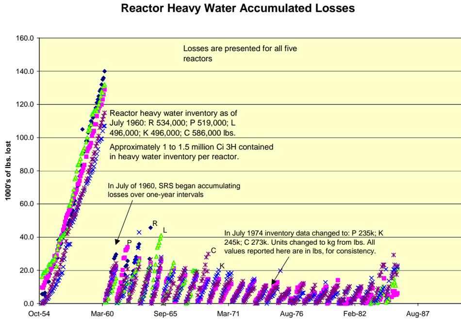
**Figure 2-10.** Because reactor heavy water moderator was an expensive SRS product, its loss rate was monitored routinely. Tritium (as tritiated water) was present in the moderator and was released offsite via moderator leakage. Routine tritium loss from the reactors may be estimated using records of moderator loss ([Du Pont XX](#)).
