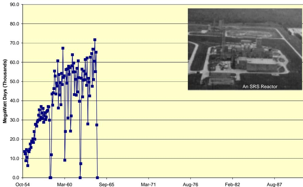
**Figure 2-5.** R-Reactor operated from December 1953 to June 1964, initially reaching 375 MW thermal power. Modifications increased power levels over time. R-Reactor reached its maximum of 71,700 MWd in March 1964. The reactor developed significant vessel cracks, discovered in mid-1960 ([Du Pont XX](#)).
