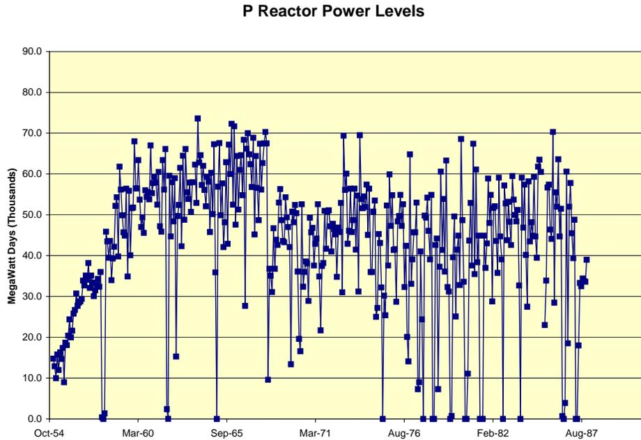
**Figure 2-6.** P-Reactor operated for nearly 35 years, reaching its maximum monthly power output of 73,600 MWD in December 1963 ([Du Pont XX](#)).
