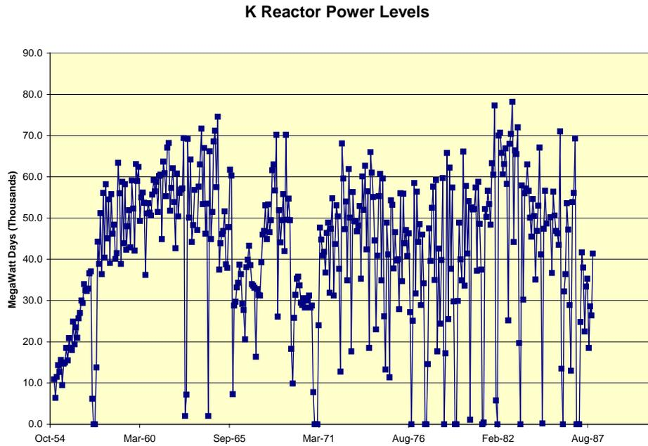
**Figure 2-8.** K Reactor operated for more than 30 years, reaching its peak monthly power output of 78,200 MWd in January 1983 ([Du Pont XX](#)).
