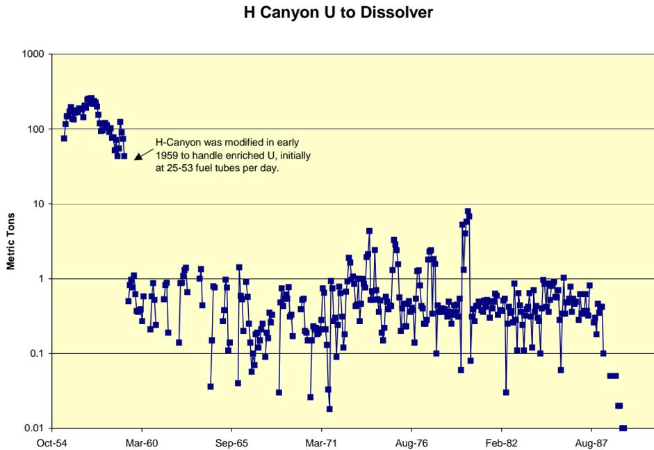
**Figure 2-12.** H-Canyon uranium to dissolver. In later years, H-Canyon throughput was reported both in metric tons of heavy metal (uranium) and as the number of (enriched)  $^{235}\text{U}$  tubes charged to the dissolvers ([Du Pont XX](#)).
