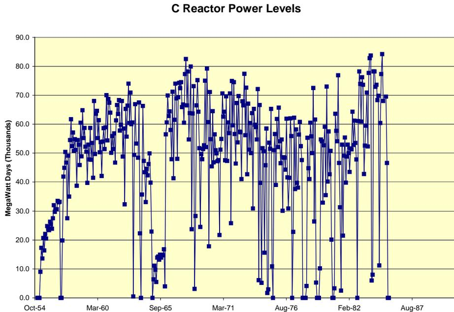
**Figure 2-9.** C-Reactor also operated for more than 30 years, reaching a peak monthly power output of 84,200 MWd in January 1985. Inspections in the early 1960s indicated cracking in a highly stressed section of the vessel. In 1985, additional cracks caused by helium embrittlement were found ([Du Pont XX](#)).
