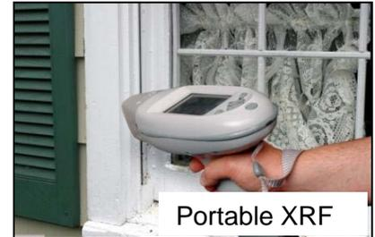
Instructor Note: Picture from Niton the manufacturer. Transporting XRF instruments across international boundaries may require additional approvals because of the cobalt source in the instrument.
