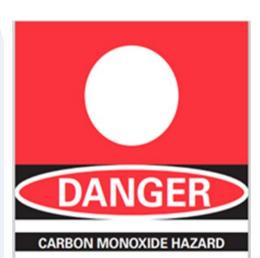
Using a generator indoors WILL KILL YOU IN MINUTES. Exhaust contains carbon monoxide, a poison gas you can not see or smell.
