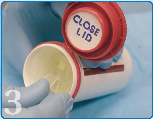
3 Put on powder-free gloves before handling cuvettes. Keep cuvettes in humidity-controlled container until ready to use. Recap the container immediately after withdrawing a cuvette.
