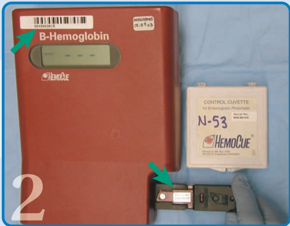
2 Check the instrument for accuracy using the instrument-matched calibration cuvette (arrow). If the calibration cuvette provides a reading that is not within the range specified on its container, clean the cuvette holder and the cuvette with a dry, lint-free wipe. If the cuvette reads within the specified range, perform one of the daily quality control (QC) tests on the instrument.
