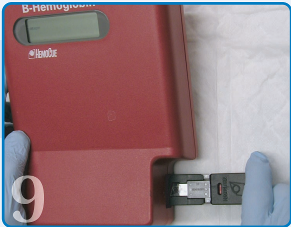
9 Place the cuvette in HemoCue® instrument. Gently push the holder into the photometer. Record the result.
