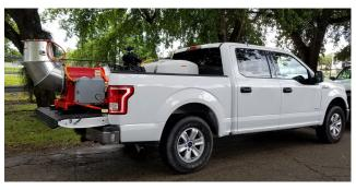
Mosquito control truck used for spraying larvicides like Bti.
