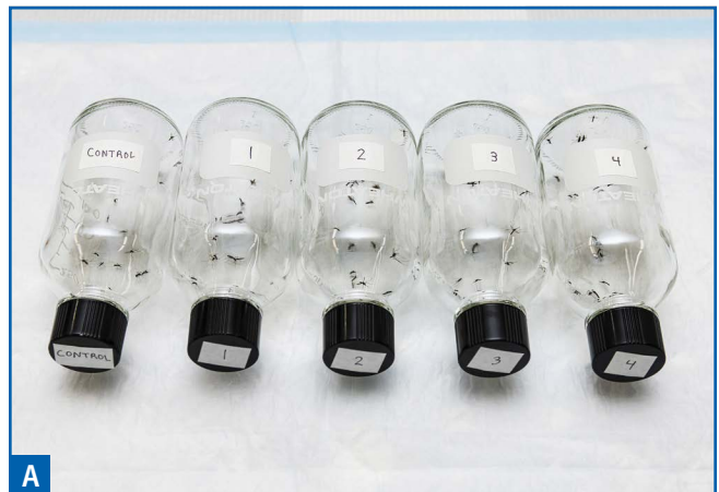
Figure 8: CDC bottle bioassay in progress. Bottles can be kept horizontally (A) or vertically (B).
