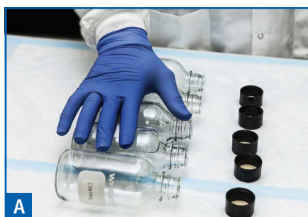
Figure 6: Drying the bottles manually (A) or with a bottle roller (B).
