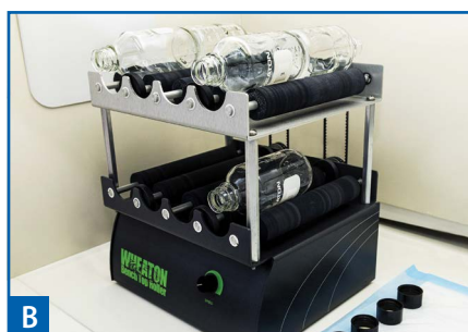
Figure 6: Drying the bottles manually (A) or with a bottle roller (B).
