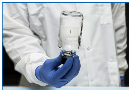
Figure 4: Coating the inside of the cap.
