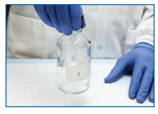
Figure 4: Coating the inside of the cap.
