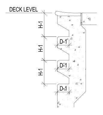
Figure 4.5.7.4.2: Recessed Step Dimensions
