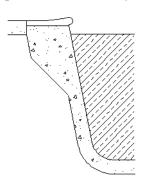
(C) Structural support ledge all within 1 in 5 slope.
