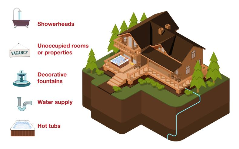
**Showerheads:** *Legionella* can grow in and spread through showerheads if they have not been used regularly (e.g., a week or more), if they have not been replaced or cleaned in a long time (e.g., there is visible buildup on the aerators), or if there are low disinfectant levels in the water.
