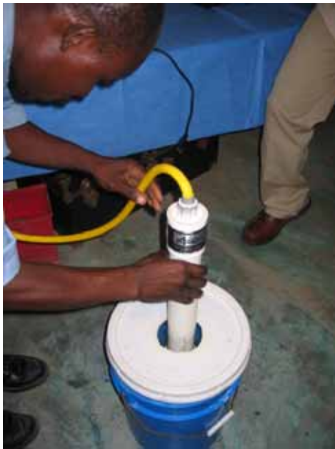
It takes approximately 2 hours to turn 17 liters of brine into 17 liters of hypochlorite solution
