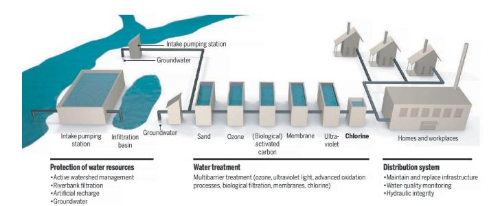
Figure 1: Drinking water system. This figure illustrates the path water takes from water source, to water treatment, to water distribution system.
