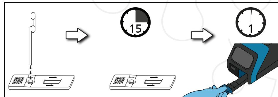
Add the correct amount of specimen to the test device as indicated on the pipette. Incorrect pipette technique such as bubbles in the pipette may lead to insufficient specimen volume.
