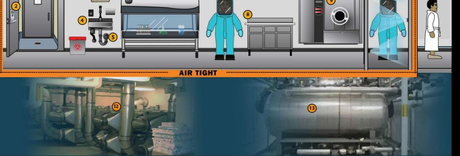
physical containment device positive pressure protective suit 8 laboratory bench 🧕 autoclave chemical shower out personal shower out supply and exhaust HEPA filters effluent decontamination system B
