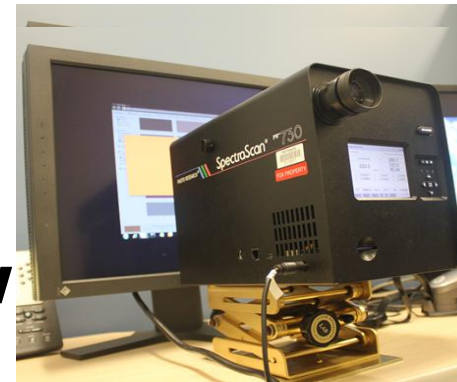
Spectroradiometer and results for grayscale tracking using different color calibration kits (adapted from Suarez et al., Proc Electronic Imaging, SPIE, 2012).
