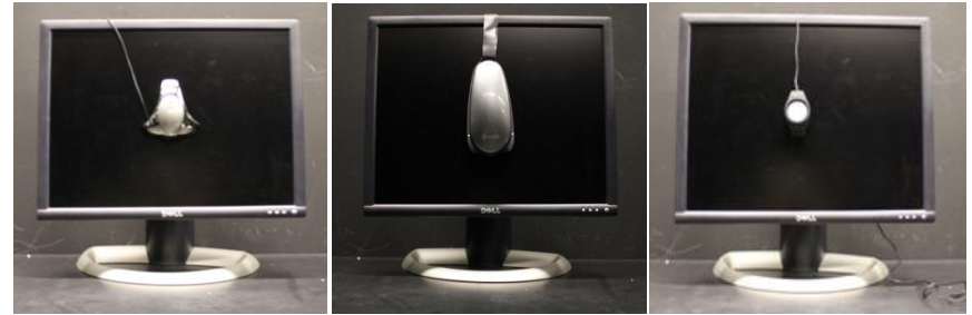
Three color kits being tested in FDA's display evaluation laboratory (adapted from Cheng and Badano, Proc SID, 2011).
