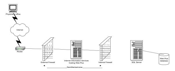
A router connects the demilitarized zone to the Internet. A Secure Sockets Layer (SSL) digital certificate is installed on the web server for site authentication and encryption of data transferred between the clients and the web server. The digital certificate can be created internally if a certificate server is available, or it can be purchased from a vendor. If the organization does not have a registered Internet domain, it needs to register one.
