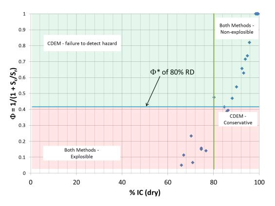
Figure 4. Comparison of CDEM results and lab TIC results for one representative mine.
