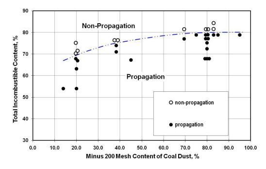
Figure 1. Effect of particle size of Pittsburgh seam bituminous coal dust on the explosion propagation for % TIC as tested within LLEM [NIOSH 2010]. The dashed curve represents the propagation/nonpropagation boundary.
