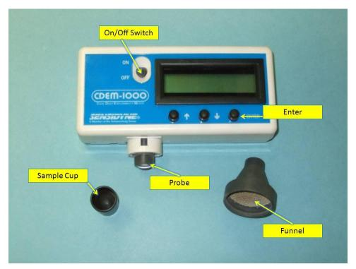
Figure 2. Coal Dust Explosibility Meter (CDEM).
