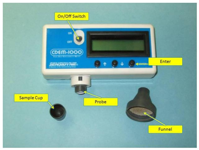
Figure A1. Coal Dust Explosibility Meter (CDEM).
