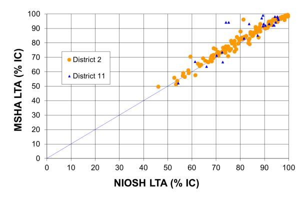
Figure 7. Comparison of MSHA and NIOSH incombustible measurements [Harris et al. 2008].
