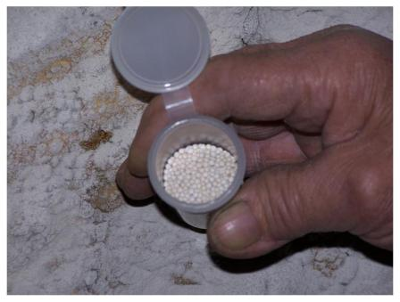
Figure C1. Sample tube containing molecular sieves.
