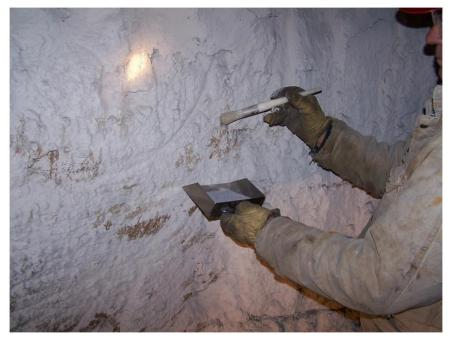
Figure C2. Collecting a band sample.
