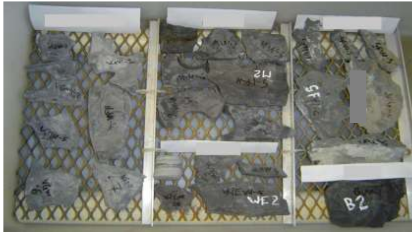
Figure 3: Roof rock samples before water immersion cycling test.
