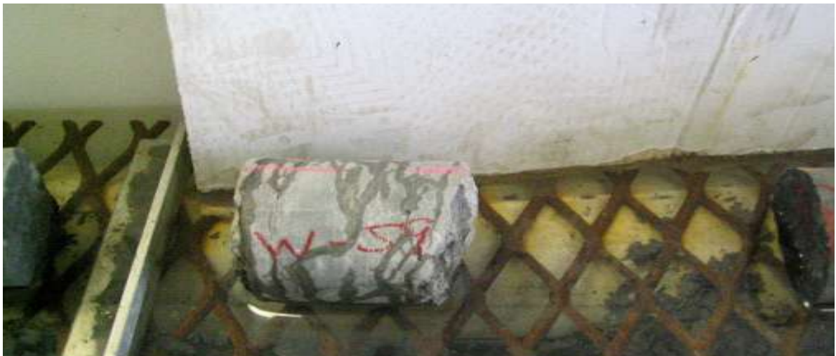
Figure 8: Fireclay showing disturbed bedding and water moving easily on bedding.
