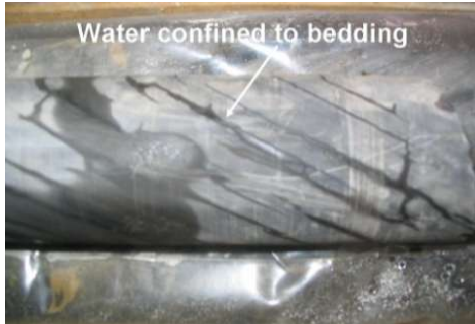
Figure 6: Water moves more readily along bedding than across bedding.
