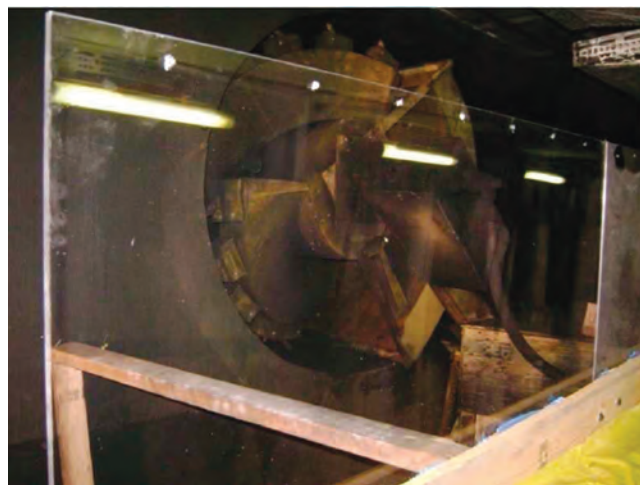
View of headgate cutting drum through partial barrier.
