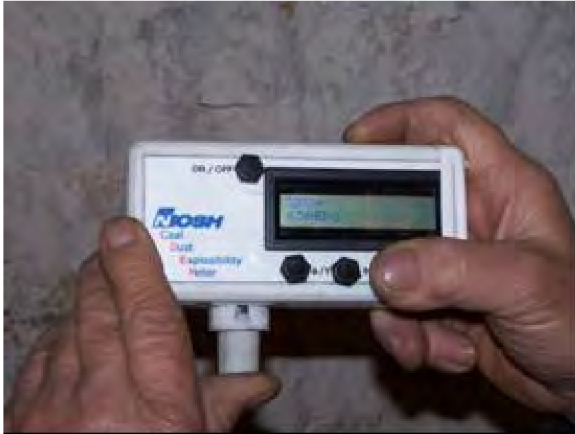
Figure 7. Coal Dust Explosibility Meter
