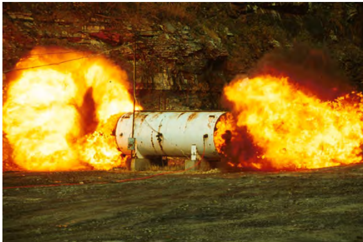
Figure 4. Coal dust ignited by explosives at the Lake Lynn Laboratory Cannon Gallery
