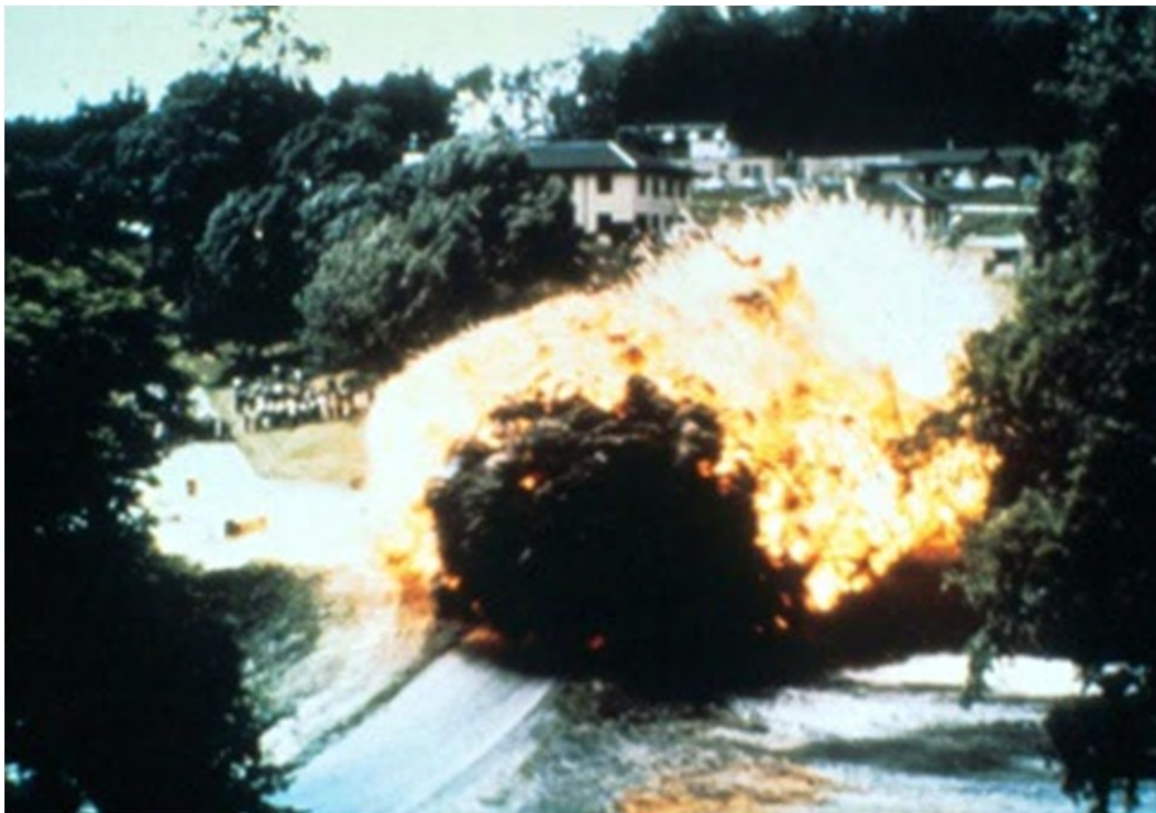
Figure 1. Bruceton Experimental Mine coal dust explosion demonstration
