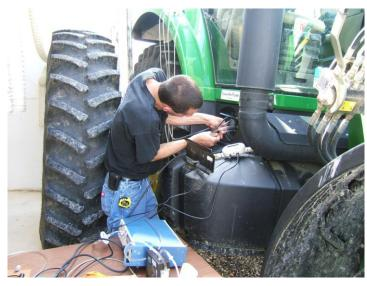
Figure 6. Leak testing the John Deere tractor cab. (Photo courtesy of Clean Air Filter).
