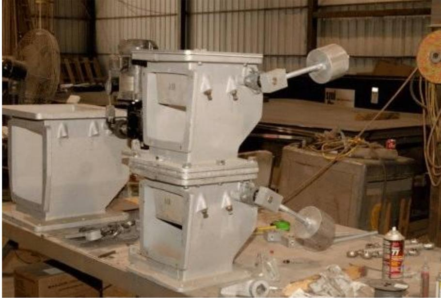
**Figure 1.24. Double dump weight-based valves.**
