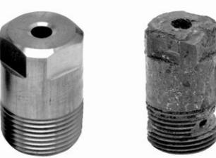
**Figure 2.18. Temperature damage—new versus used [SSCO 2004].**
