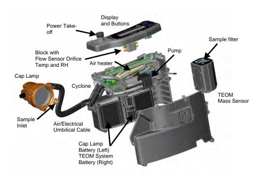
Figure 1.—PDM internal components.
