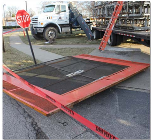
Figure 1. The cage door that fell from the flatbed trailer onto the victim.
