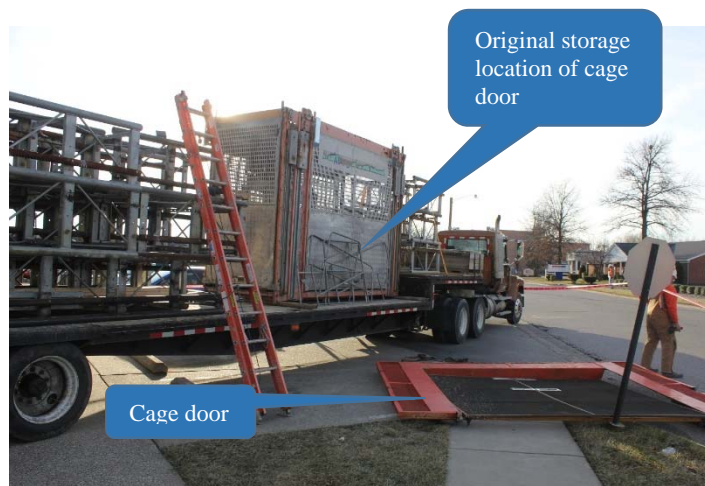
Figure 3. The cage door that fell on the victim and its original storing location.
