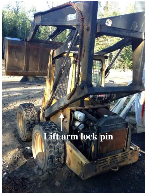
Figure 3 – Skid-steer with lift arm raised and mechanical lift arm lock engaged
