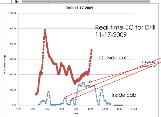
Potential open door or window causing higher DPM concentration (coincides with drops in cab pressure)
