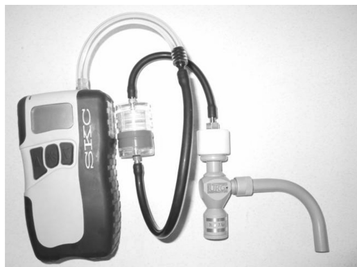
Figure 2. A high volume setup consisting of a cyclone with a 1\ \mu\text{m} cutpoint at 8 lpm, filter to collect particulate and a high flow rate (5–15 lpm) personal pump.
