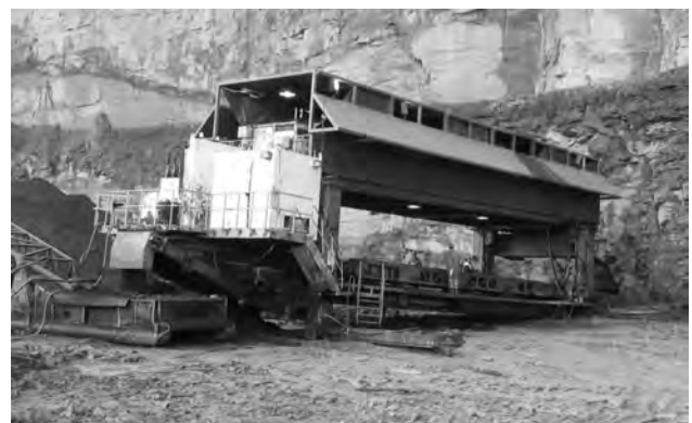
Figure 2. Addcar Highwall Miner in operation. Note Addcar in launch vehicle, control cab and discharge conveyor.
