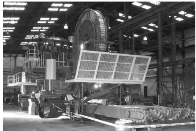
Figure 1. Superior Highwall Miner under construction. Note thin seam cutter-head, control cab and cable reel.
