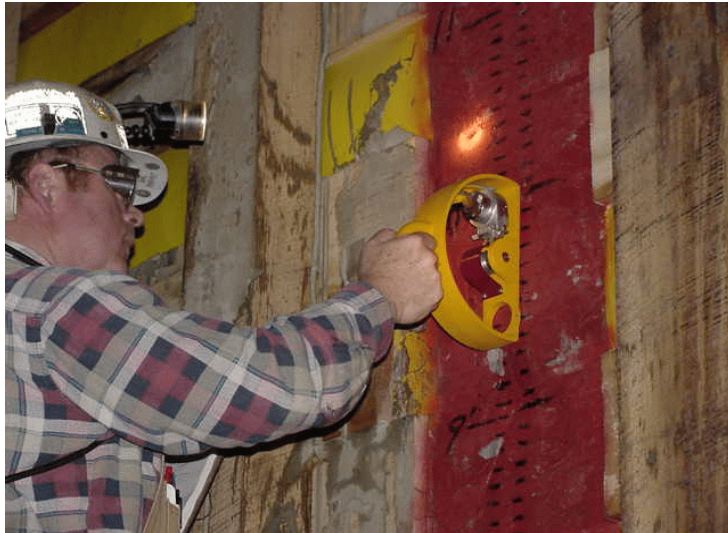
Figure 4. Miner performing Schmidt Hammer test on Section 3 of the mine seal.
