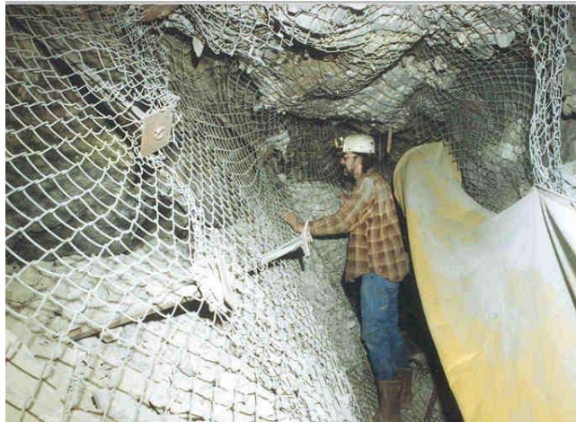
Figure 2. Underhand stope survives 3.5 ML rockburst.
