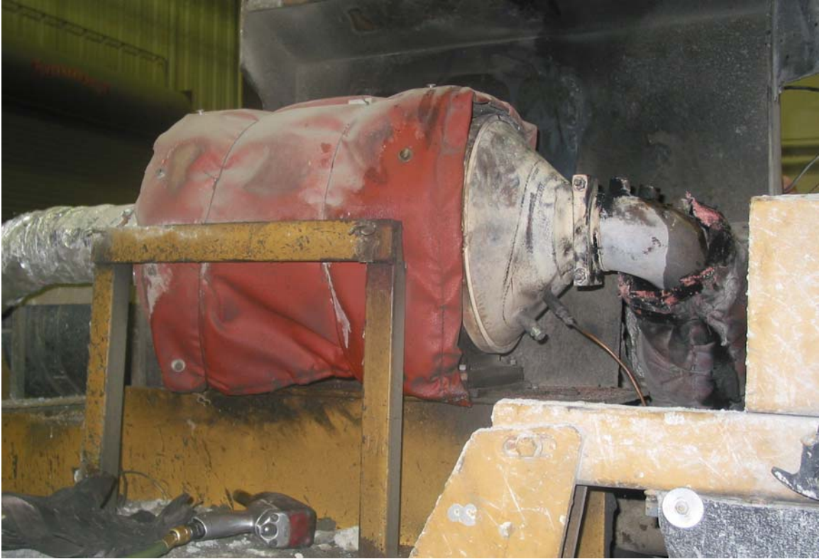
Figure 1. Engelhard DPX DPF system on the truck #92128
