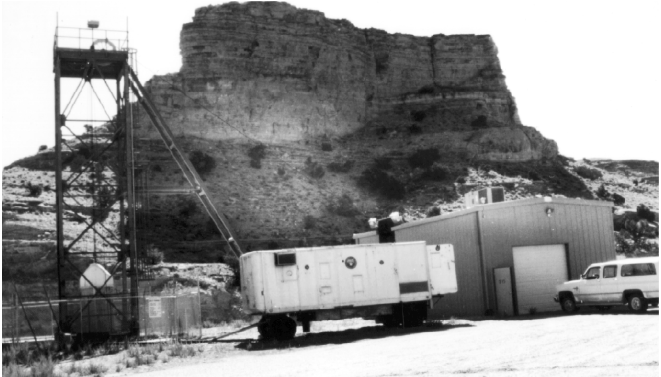
Figure 22.—Gas monitoring trailer near air shaft at White River Mine.
