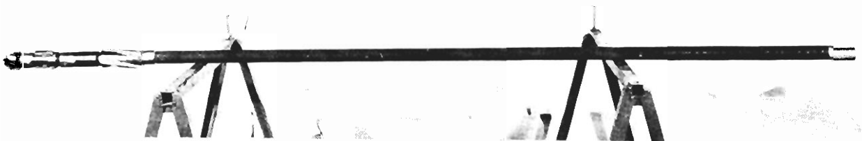
FIGURE 4. • Drill string with one centralizer behind bit.
