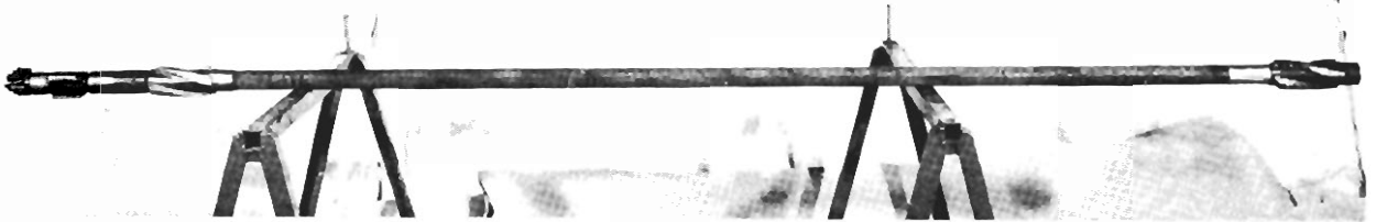
FIGURE 6. - Drill string with two centralizers 10 feet apart.
