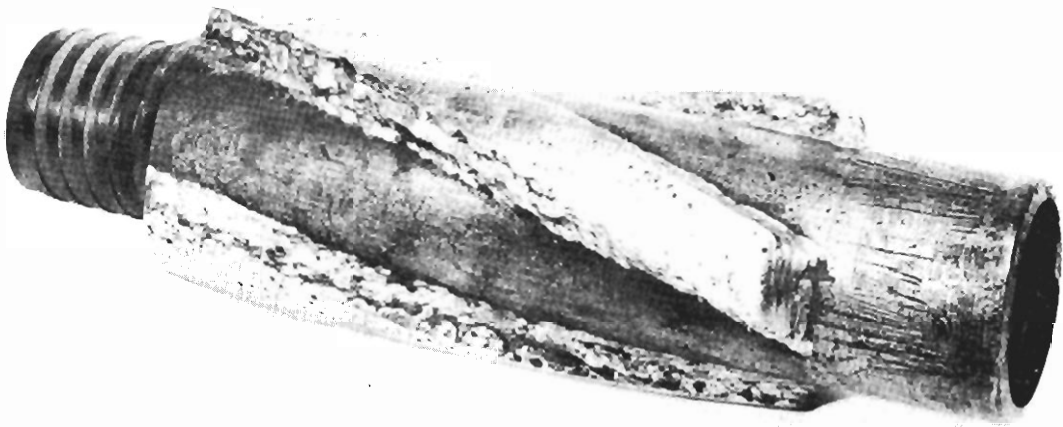
FIGURE 2. • Drill string with bit and drill casing.
