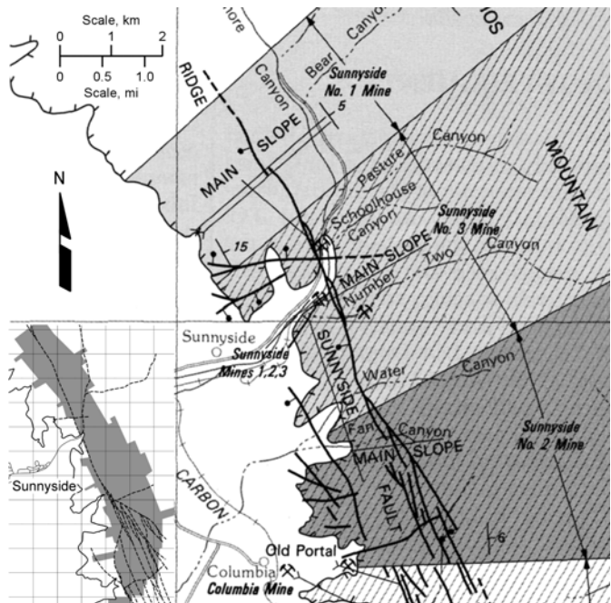
Figure 1 The main Sunnyside fault zone in the Sunnyside 1,2 and 3 Mines (after Osterwald, 1993). Inset is a map of mining to 1958. Shaded area is 4 sq. miles of worked out or first mined coal seam (after Peperakis, 1958).
