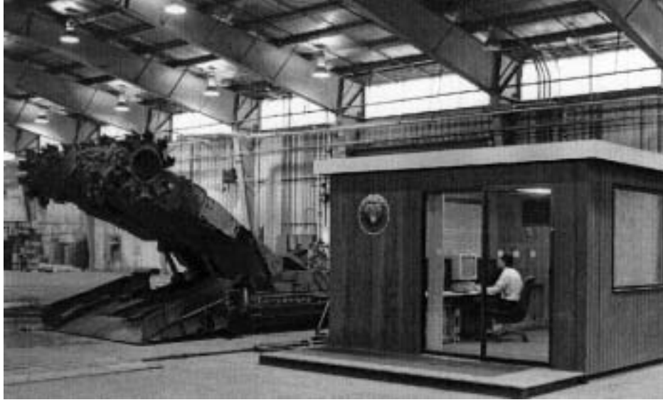
Control of a cutter from a remote location.
