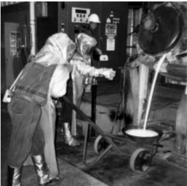
Project personnel conducting spot checks for mercury vapor during a pour of molten slag.
