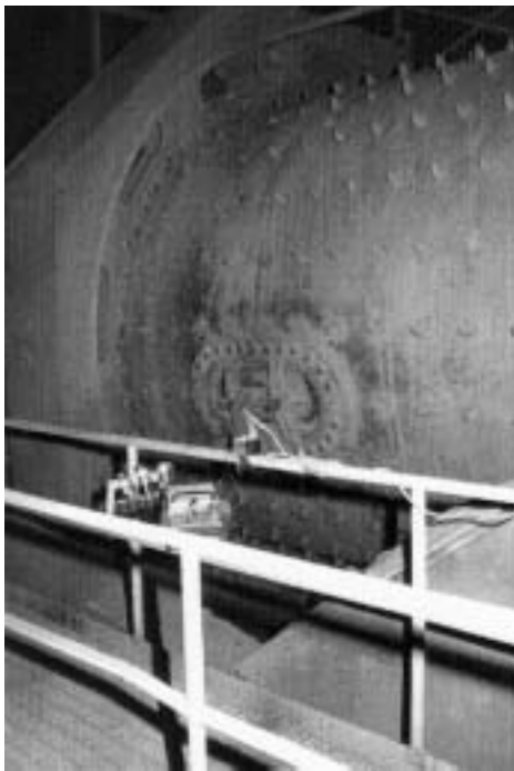
Instruments sampling respirable dust concentrations near pebble mill in portland cement plant.
