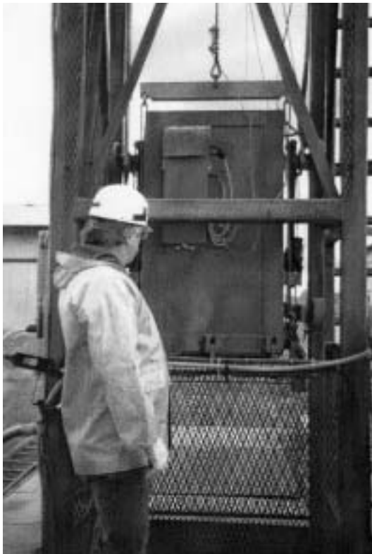
Skip inside headframe at test facility. See diagram above for location of data acquisition equipment.
