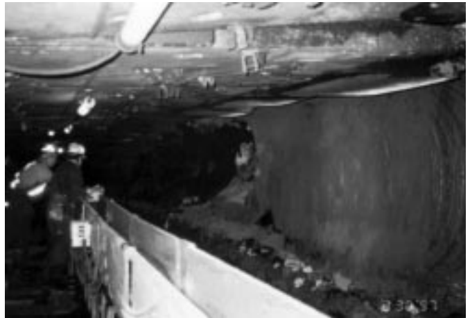
Mining through backfilled cross-panel and entry pillars in the 8-Right longwall panel at the Foield Creek Mine.
