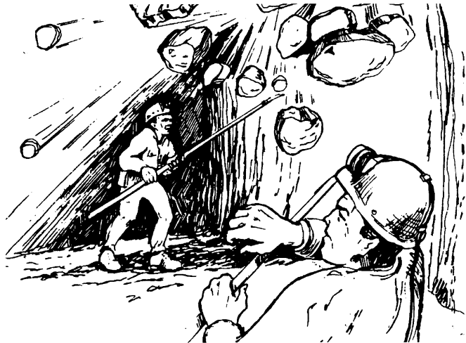
The obvious hazards of scaling loose rock.
