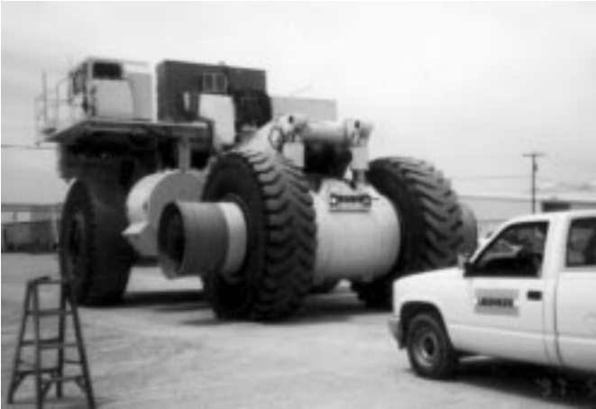
Doppler radar backup alarm being tested on 240-ton class mining truck.
